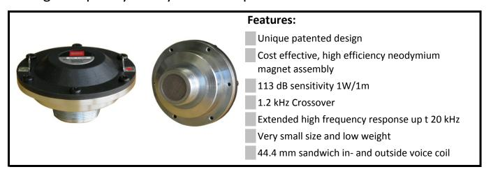
The BMS 4545ND is a powerful 1" professional compression driver that delivers superb sonic quality in a small package. The unique BMS annular diaphragm together with the cost effective, high efficiency neodymium magnet assembly offers an economical solution for a wide variety of high level professional reinforcement systems applications.
